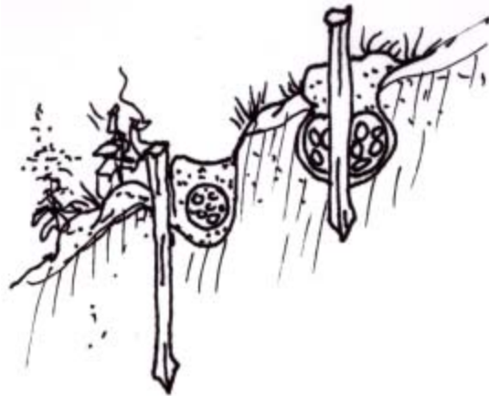
Figure 5: Anchored drains (adapted from Scheichtl 1980)
