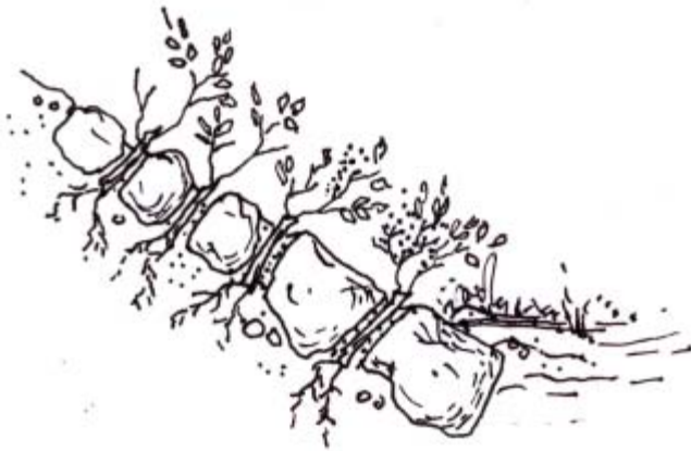
Figure 16: Joint planting (adapted from Schiechtl et al. 1980)
