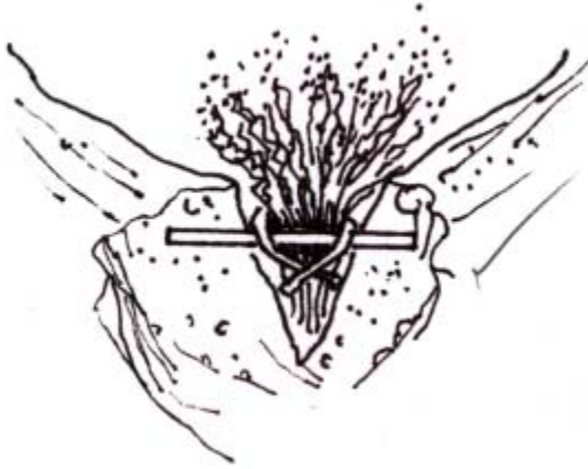
Figure 1: Anchored live branch gully (adapted from Schiechtl 1980).
