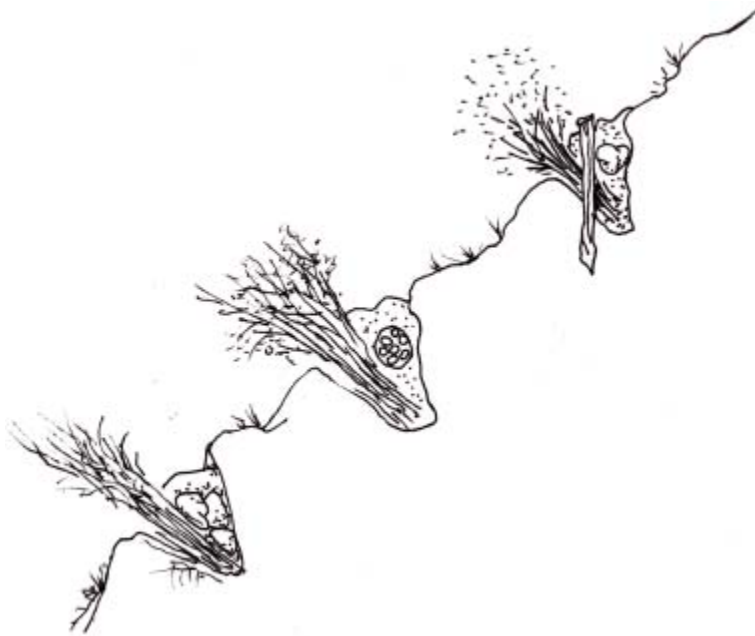
Figure 9: Variations in the brush layer method. Rooting material is stabilized with rock (left), a fascine or gambion (center), and stake and pole anchoring device (adapted from Schiechtl 1980).
