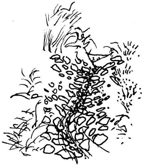
Figure 3: Rock stabilization with fascine drains (see below). (Drawing adapted from a photograph in Schiechtl 1980).
